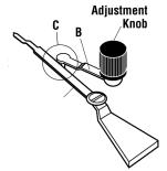
closes with the limit contact (B), a control circuit (C) is completed and signals an alarm and/or shutdown or starts/stops a pump.
